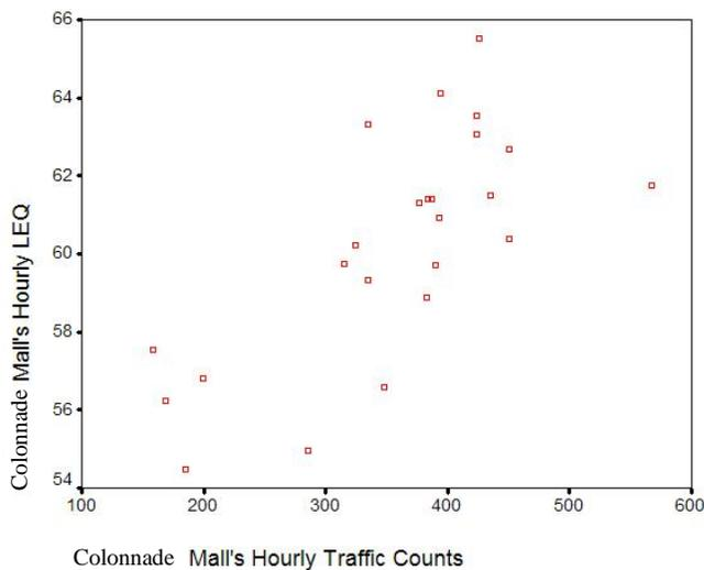
**Figure 14: Scatterplot of hourly  $L_{eqs}$  versus hourly traffic counts at the Colonnade Mall**
