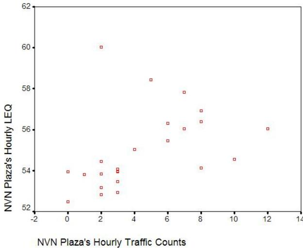
**Figure 15: Scatter plot of hourly  $L_{eqs}$  versus hourly traffic counts at the NVN Plaza**
