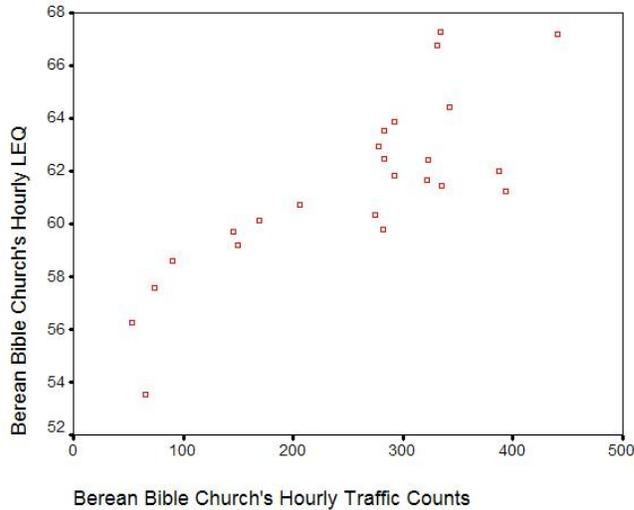
**Figure 16: Scatterplot of hourly  $L_{eqs}$  versus hourly traffic counts at Berean Bible Church**
