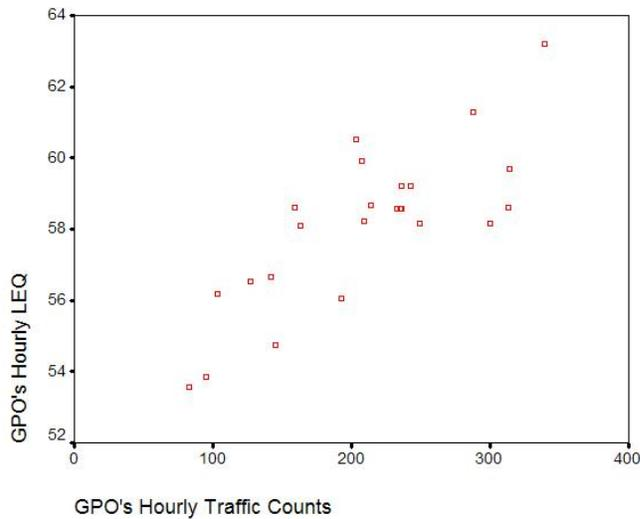
**Figure 13: Scatter plot of hourly  $L_{eqs}$  at GPO versus hourly traffic counts at GPO**
