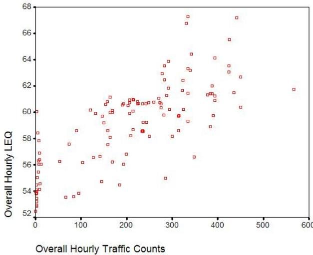
**Figure 18: Scatterplot of hourly  $L_{eqs}$  versus hourly traffic counts for all sites combined**
